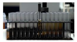
Gas infusion mixing of used oil and solvent with SampleSense *FAST* UHT-O system just prior to analysis on Agilent 5900 ICP-OES.
